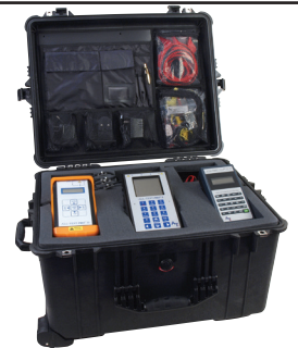
De-energized testing for troubleshooting and incoming inspection
